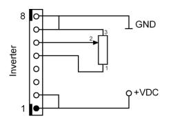
Dimming with variable analog DC voltage. Variable voltage 0 to 5 VDC (pin 7: 0 V)
