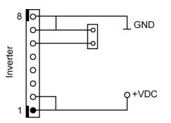
3. Digital Dimming with PWM control 0 to 100% PWM, PWM 200-1000 Hz; TTL-Level (pin 7: 0 V), recommended frequency 200Hz,
