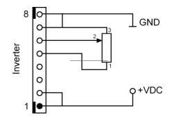
2) Dimming with variable analog DC voltage. Variable voltage 0 to 2.5 VDC (pin 7: 0 V)
