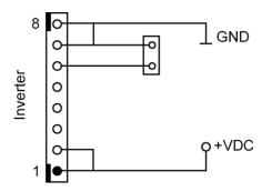
3) Digital dimming with PWM control 0 to 100% PWM, PWM 200 – 1000 Hz; TTL-Level (pin 7: 0 V)
