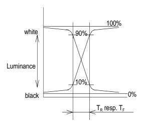
note (4): Brightness measurements setup
